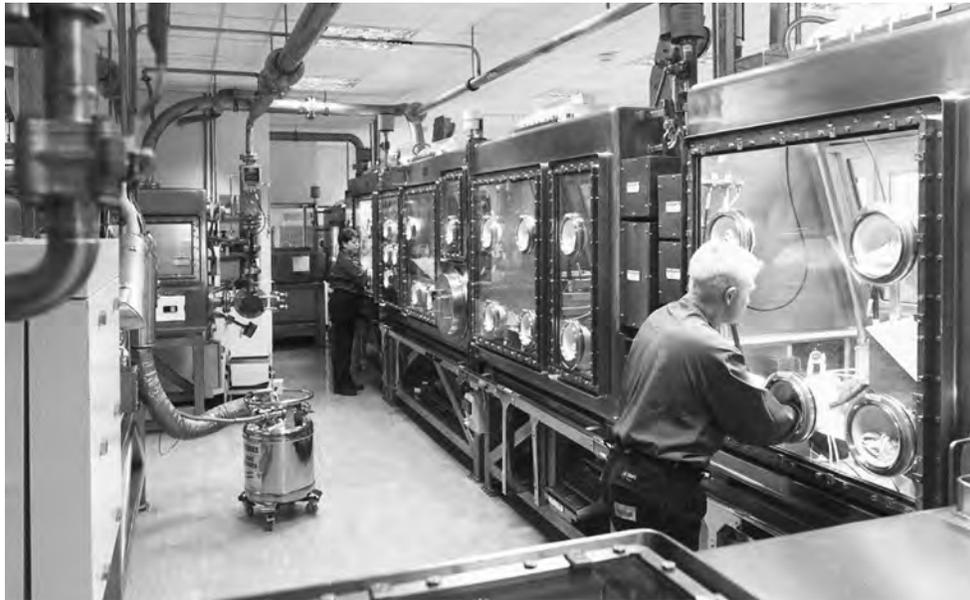
**Figure 10** Glovebox line at the former Sellafield MOX Fuel Fabrication Plant. *Source:* UK Nuclear Decommissioning Authority.
